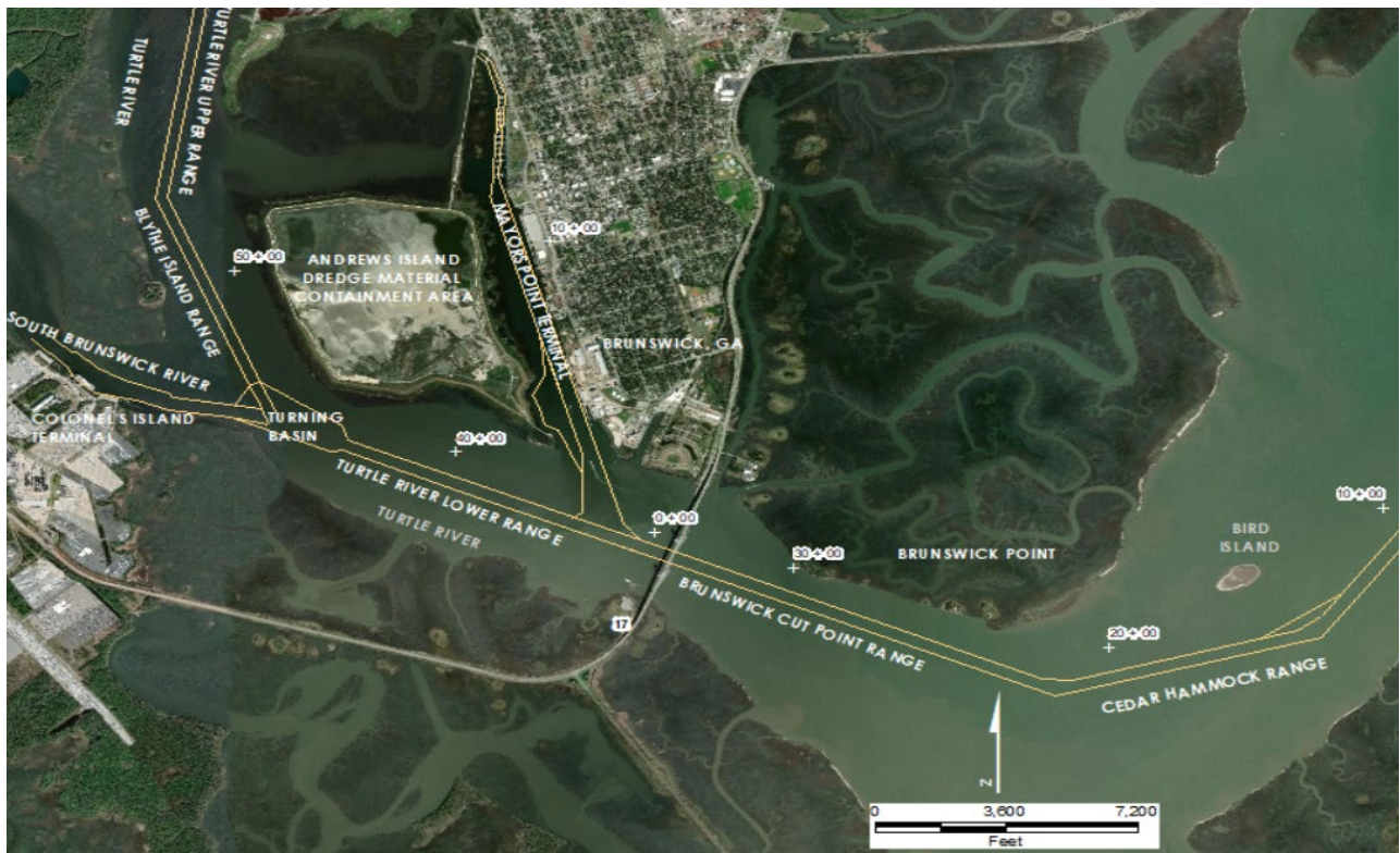
Figure 5 - Existing Inner Harbor Channel Configuration of Brunswick Harbor
