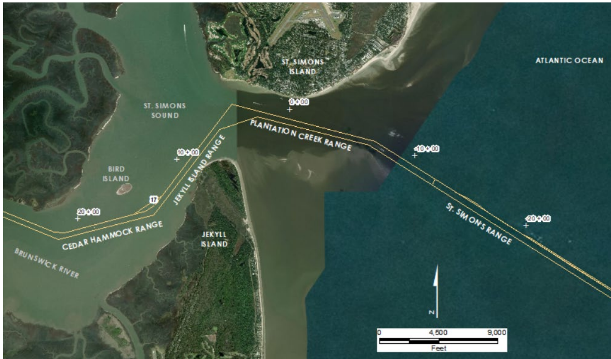
Figure 4 - Existing Entrance Channel Configuration of Brunswick Harbor
